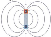
An electromagnet uses the principle that a current through a wire causes a magnetic field. Its strength depends on the current, the core and the number of coils in the solenoid.
