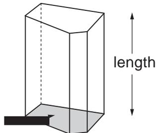
$$\text{Volume} = \text{area of cross-section} \times \text{length}$$
